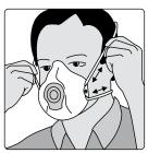
4. Adjust strap by pulling loop on strap.
